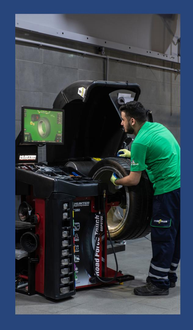
• **Attaching** the appropriate weight on the opposite side of the tire to compensate forweight differences Remounting tires and wheels.
